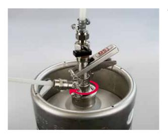
15. Reconnect the dispense head to the beverage container. Push the dispense heads A-type and combi onto the disc of the spear respectively turn the dispense heads S-type, G-type and Draft into the spear clockwise.
