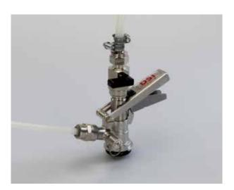
14. Refit and tighten the hose connections to the dispense head and refit the respective hoses.
