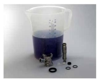
9. Lay the single components of the dispense head in a cleaning agent and disinfectant and allow it to react (reaction time prescribed by the agent).
