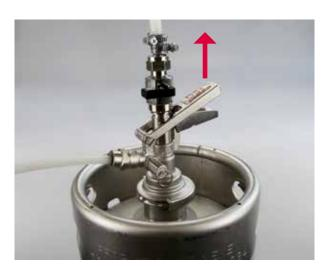
2. Disconnect the dispense head from the beverage container. If there is a ball valve on the piston close the beer line.
