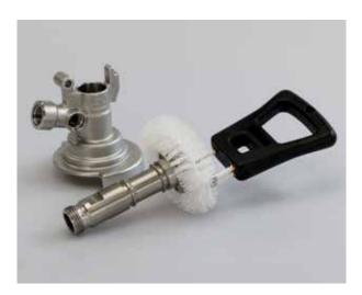
10. Brush the bodies S-type and Draft as well as the corresponding pistons with the cleaning brush (article-no. 550396). Brush the bodies A-type, G-type and combi as well as the corresponding pistons with the cleaning brush (article-no. 550395). Rinse all components with clean water.
