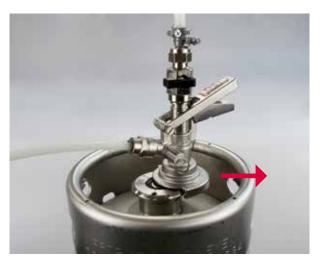
3. Pull dispense heads A-type and combi from the disc of the spear respectively or in the case S-type and G-type, turn the dispense head anti clockwise to release it from the spear.
